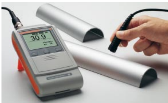
DUALSCOPE® FMP20 with anodized parts. Measured using the patented curvature-compensated probe FTD3.3
