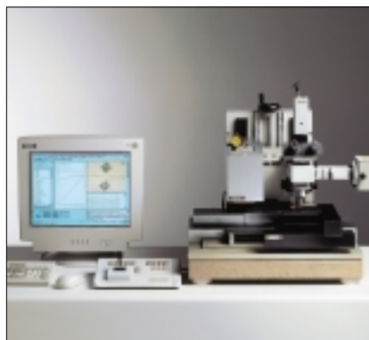
Micro hardness measurement unit FISCHERSCOPE® H100 to determine the universal hardness HU of thin coatings and foils.
