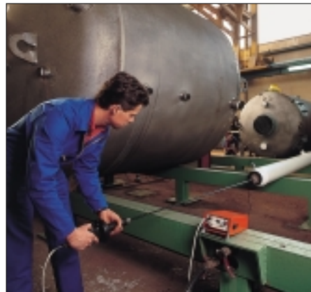
Test of the interior coating of a pipe with the POROSCOPE® HV20 using a rotating electrode on a rod extension system.
