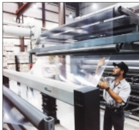
Five-coating stretch-foil casting plant of the SMS Company, Texas/USA.
